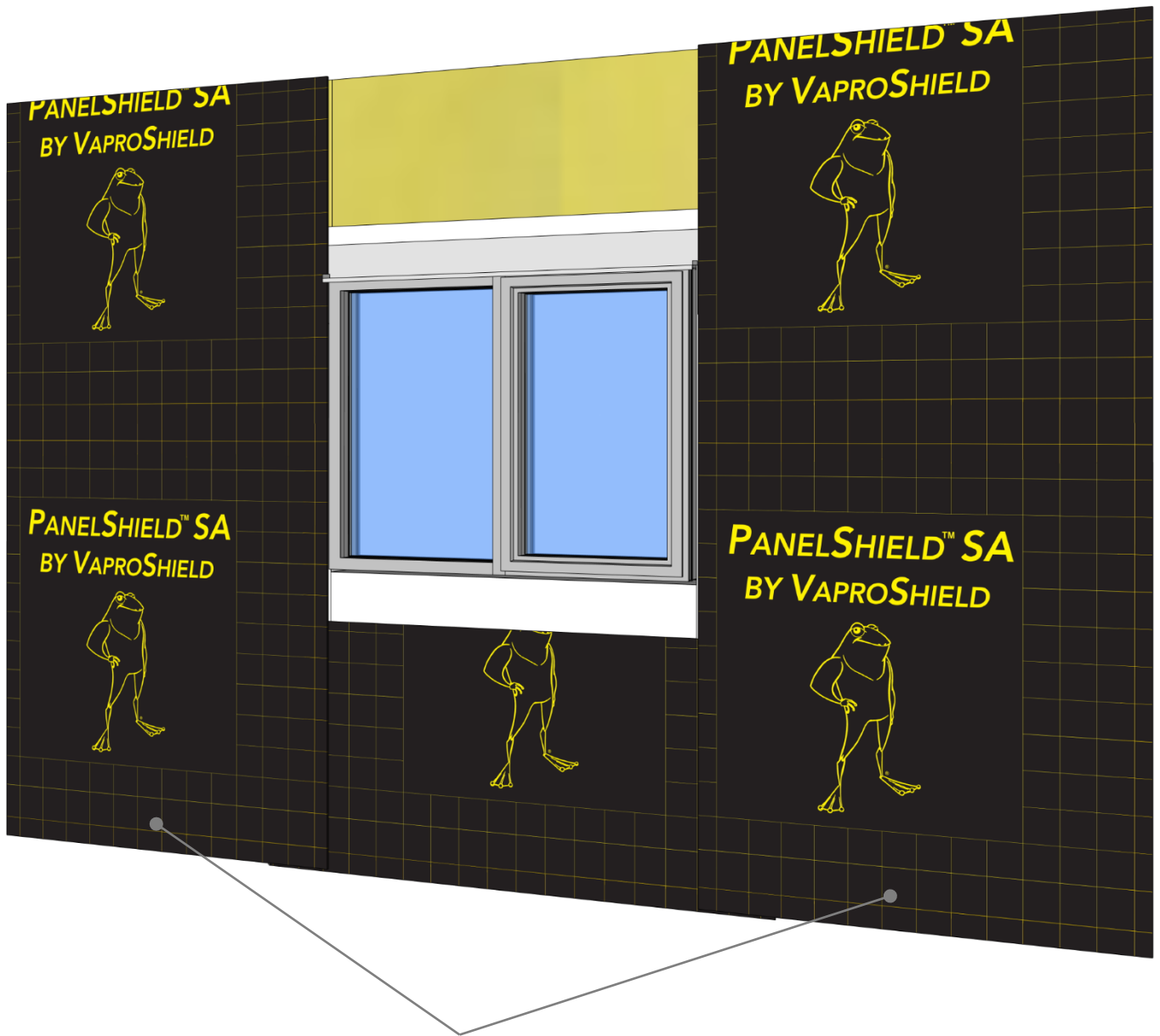
PanelShield SA Self-Adhered field membrane installed with minimum 3" overlap
